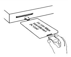
The perfect solution for your laptops to high speed LAN through the PC Card. Now it comes true for the laptop users to hook up to their Ethernet LANs at the speed of 100Mbps which is 10 times faster than traditional LAN environment. Moreover, the support of full duplex mode makes the data rate double possible. The fantastic feature of 10/100M auto-negotiation cleans away the backwards compatible troubles.
